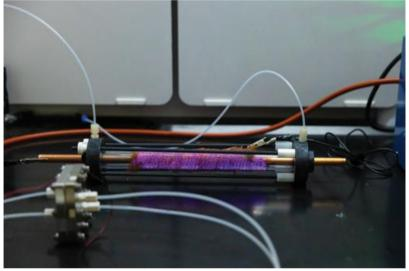
mixture is fed to an electrochemical reactor, where the NOxHy compounds are selectively converted into ammonia. The team has stably operated a reactor system producing around 1 g/day of ammonia for over 1,000 h.
