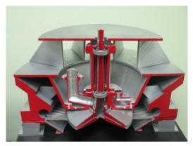
Eirex's process introduces a necessary cavitation-generating turbulence into an accelerating, dynamically pressurized feedstock, such as heavy crude oil, bitumen, oil sands or petroleum refinery streams. Such a dynamic excitation creates areas of low pressure within the fluid, leading to the formation of multiple bubbles. These bubbles then violently implode. generating extremely high, localized temperatures accompanied by intense shock waves. Eirex's rotor-disintegrator
