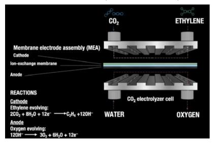
oxygen evolution reactions. Unlike most waterelectrolysis systems, CERT's catalysts do require not any precious metals. CERT's technology is designed to be agnostic to the source of CO<sub>2</sub>, that meaning industrial emissions or atmospheric CO<sub>2</sub> can be successfully converted into ethylene.
